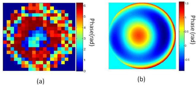
Figure 5. Phase map of the interferometric focusing (a) and wavefront measurement from SHWS (b).
