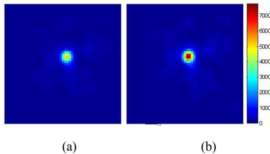
Figure 6. Images of the microsphere before (a) and after (b) wavefront correction.
