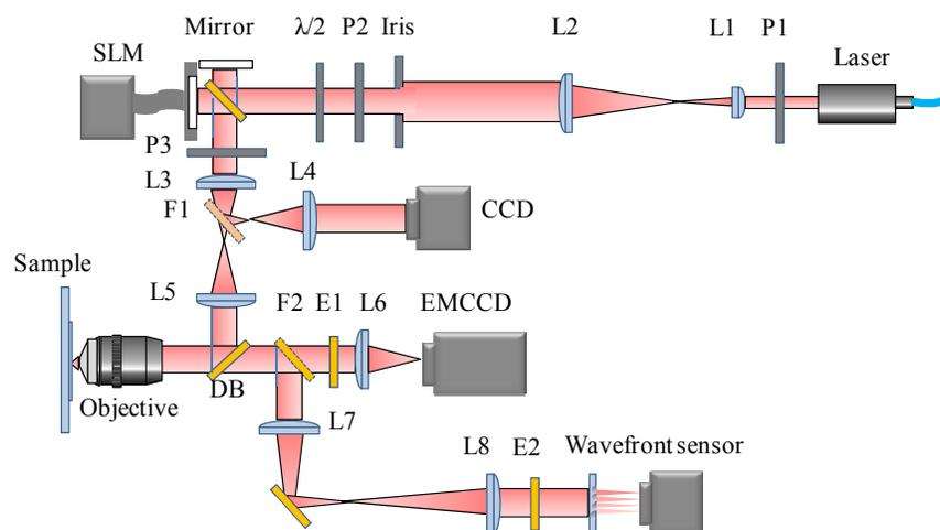
Figure 1. System Layout. L, lens; F, flipper mirror; P, polarizer; DB, dichroic beamplitters; E, emission filter.
