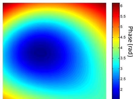
Figure 3. The phase error induced by SLM.
