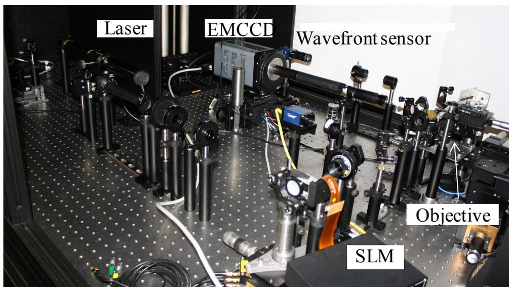
Figure 2. Experimental setup. The system was mounted on an optical table with vibration isolation.
